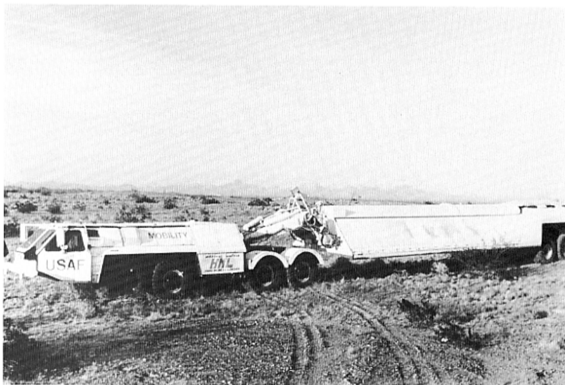
Another weapon designed for nuclear warfighting was the Midgetman small Intercontinental Ballistic Missile (ICBM), to be carried in the Hard Mobile Launcher (HML) shown here. Midgetman was de-
