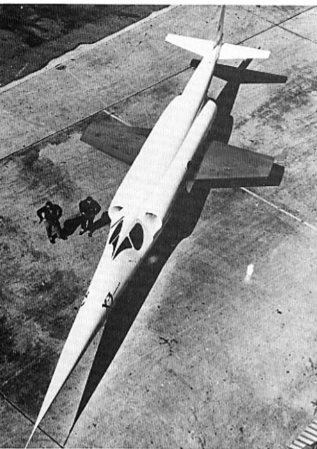
The aggressive pursuit of speed in the post-war era is typified by the Douglas X-3. Designed in 1945, when the official world's air speed record still stood at 469 mph, the X-3 was intended for sustained flight
