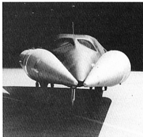
The FDL-5 was designed to be air-launched from a B-52. Fuel for initial acceleration was to be carried in two conformal tanks forming a V-shaped collar around the vehicle. USAF via David Selegan
